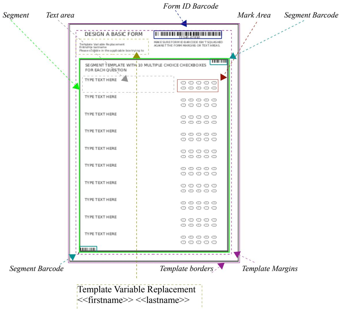
**The Form Template:** is designed using the form editor (New Form button). A form template is made up of a number of components, which all must fit within the form template's margins.
